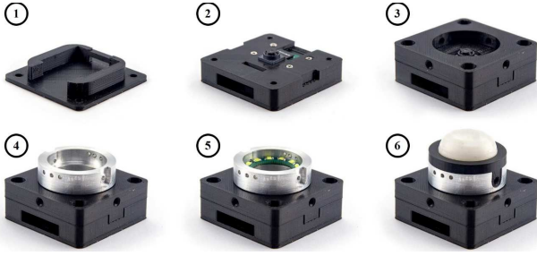
Fig. 10. Assembly steps of the fabricated sensor
