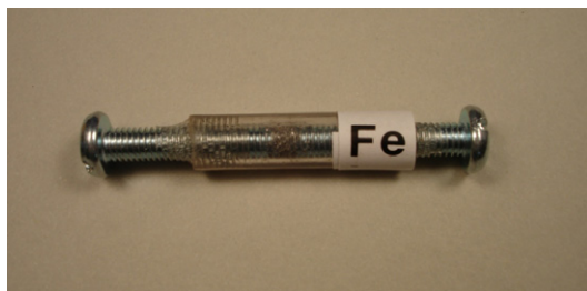
Figure 2. A simple coherer.
