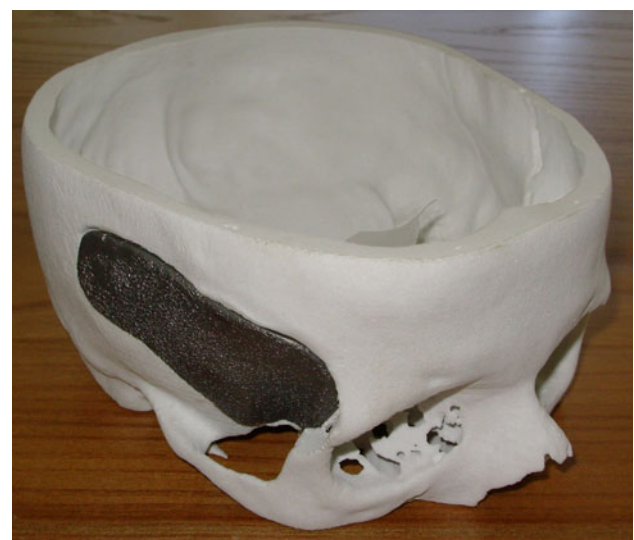
Fig. 3 Custom-made skull plate manufactured in medical-grade titanium using SLM technology
