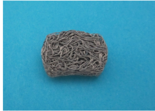
Fig. 1. Knitted disc prosthesis for cervical spine made of titanium filaments and pressed into the shape.
