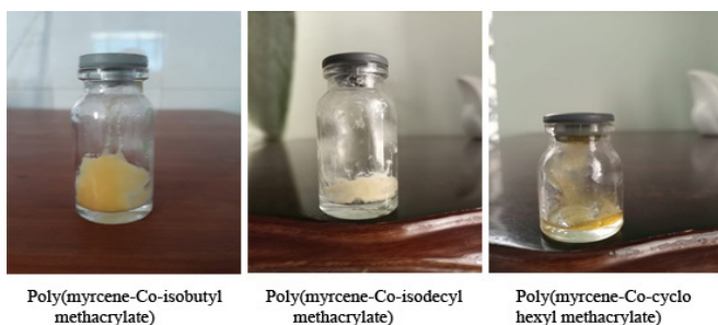
Figure 1: Photographs of the three copolymers synthesized by emulsion polymerization
