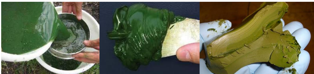
Figure 18. Concentrated suspension of microalgal biomass; a still humid paste and a more concentrated dry paste.
