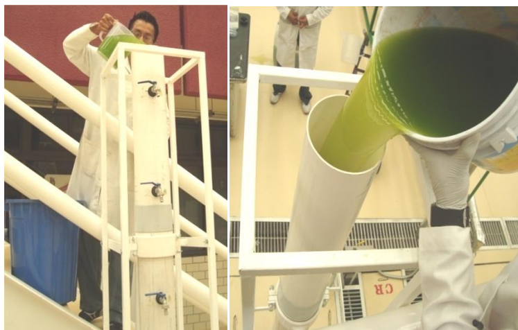
Figure 15. Thirty-eight liter column for the measurement of microalgae sedimentation rates. Photo: L. G. Torres.
