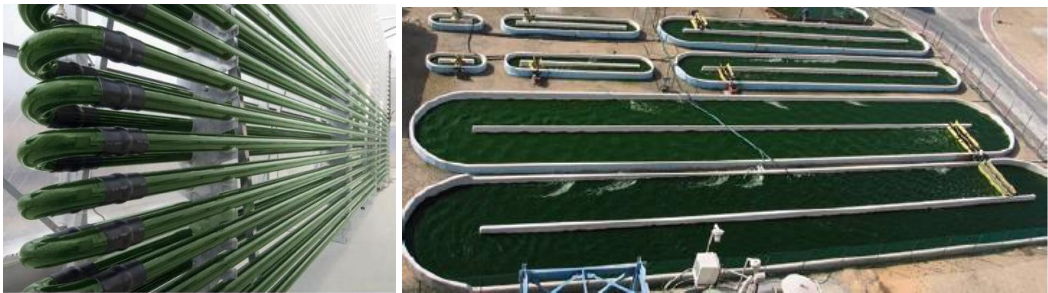
Figure 1. Closed and open systems for microalgae massive culture (left, tubular reactor; right, raceways,).
