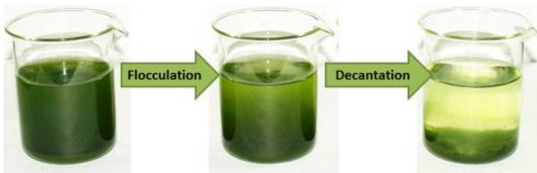
Figure 8. CF process applied to microalgal suspension.
