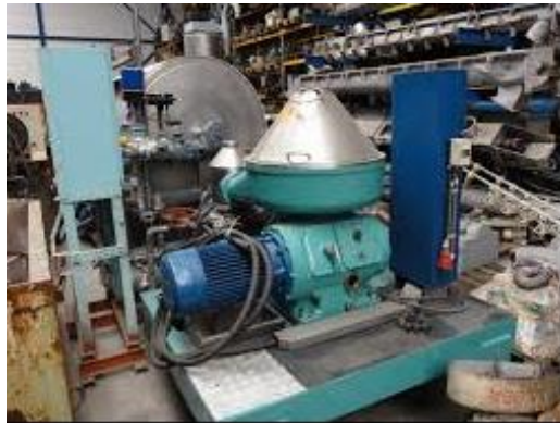
Figure 3. Common centrifuge for biomass recovery.
