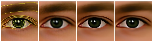
Figure 5: from left to right: raster image with the detected edges; bilinearly interpolated image; crisp edges; smoothed out edges.
