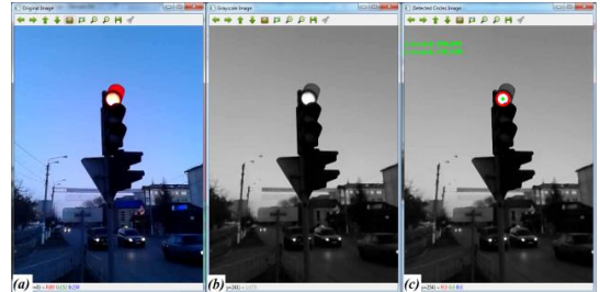
Fig. 3. The example of red traffic light circle shape detection using conversion of the original image (a) into grayscale image (b), and blurring it and displaying the circle shapes found (c) by the Hough Circles method
