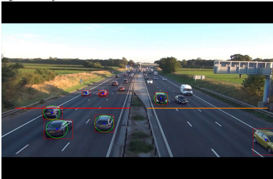
Fig.5 Counting vehicles crossing reference lines.
