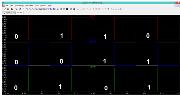
Fig. 12. Simulation of XOR gate with improved input values
