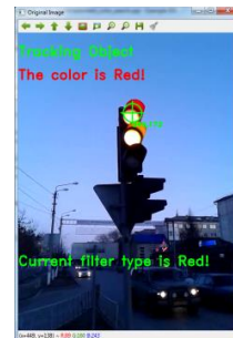
Fig.8. Example of misinterpreting traffic light signal when both red and yellow color signals displayed
