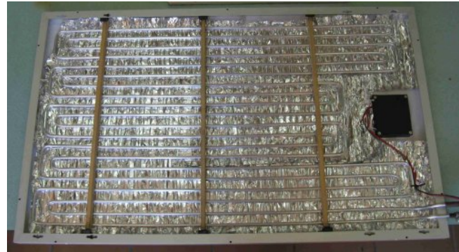
Figure 4 – View of the cooling part of the PV/ T panel
