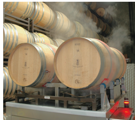
Steam treatment equipment used for the steam portion of the barrel study.
