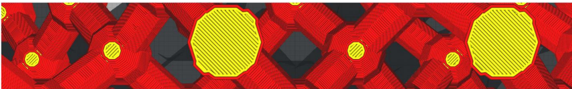
Figure 4.4: Example of unit cell lattice structure with two levels of designable mesostructure. Level 1 is the arrangement of the unit cells (red) and Level 2 is the shell-infill structure (yellow) within each unit cell element.
