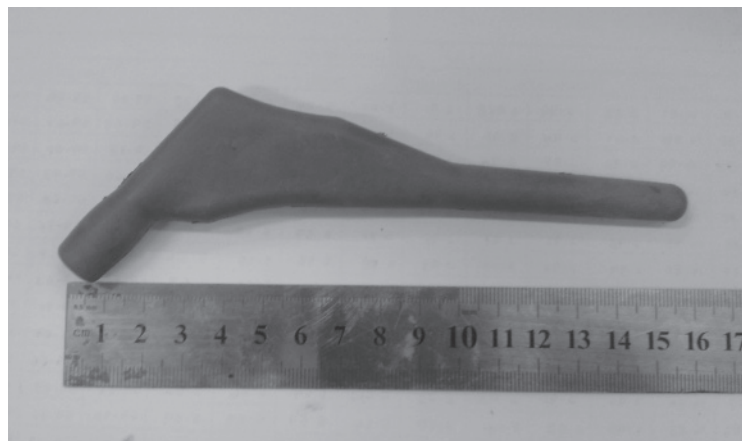
Fig. 4 Injection moulded of hip stem
