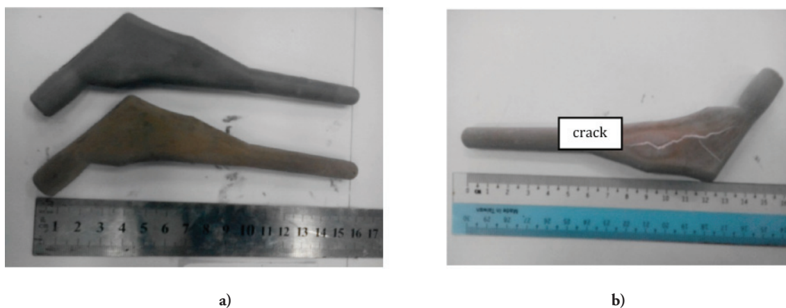
Fig. 6. a) Comparison of dimensions of hip stem after solvent extraction and thermal pyrolysis. Test samples subjected to heating rate 0.1°C/min at temperature 450°C for 1 hr show no defects. b) Thermally debound test sample subjected to heating rate 1°C/min at temperature 450°C for 1hr shows swelling and cracks
