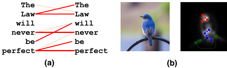
Fig. 10 Self-attention examples. a Self-attention in sentences, b self-attention in images. The first image shows five representative query locations with color-coded dots with the corresponding color-coded arrows summarizing the most-attended regions. (Color figure online)
