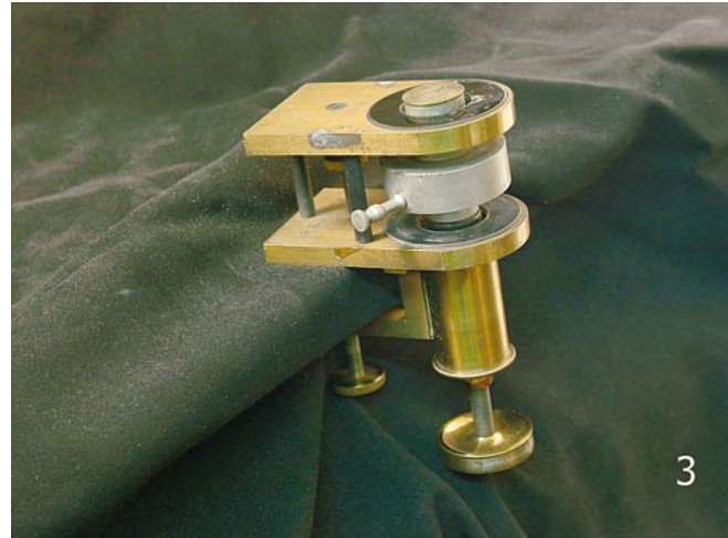
Figure 3. Freezing microtome manufactured by R & J Beck, circa 1865, used by Woodward at the Army Medical Museum (Washington, DC).
