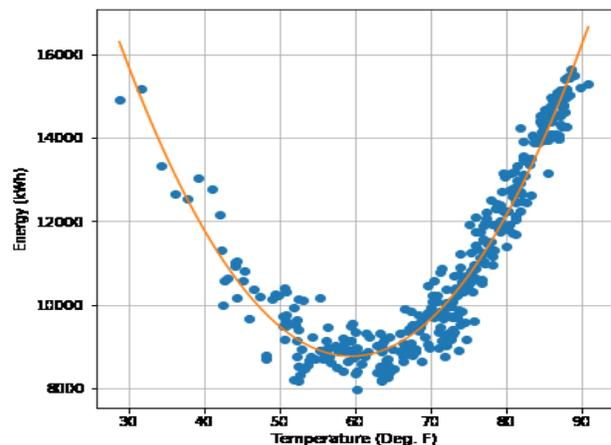
Fig. 2. Energy vs. Temperature (EvT) curve
