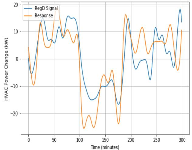
Fig. 8. Response of aggregated HVAC units to RegD signals
