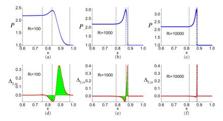
**Figure 2.** Profiles of physical quantities for different relaxation times. (a)-(c) are for the pressure P. (d)-(f) are for the corresponding non-equilibrium quantities  $\Delta_{2,xx}$  (From Ref. [22] with permission).
