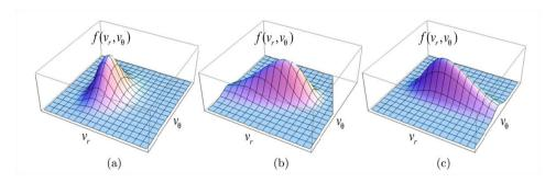
**Figure 7.** Sketches of the actual distribution functions in velocity space  $(v_r, v_\theta)$ . Panels (a)-(c) show the recovered distribution functions at the rarefaction wave, the material interface, and the shock wave, respectively (From Ref. [25] with permission).
