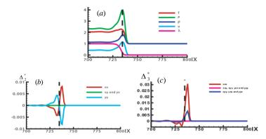
**Figure 1.** Profiles of physical quantities for CJ detonation. (a) is for the density  $\rho$ , pressure P, temperature T, x-component of velocity u, and the reaction process  $\lambda$ . (b) and (c) are for the non-equilibrium quantities  $\Delta_2^*$  and  $\Delta_3^*$ , respectively (See Ref. [21] for more details).
