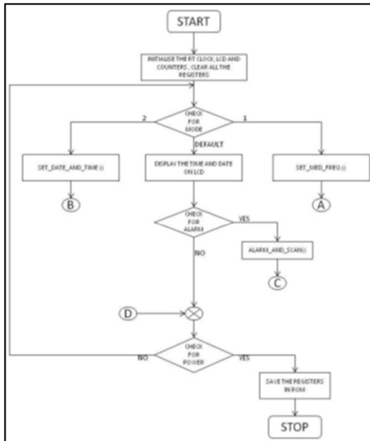
Figure 1. Flow Diagram of Working of Smart Pill Box [8]
