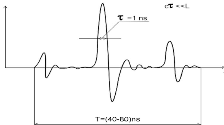
**Fig. 2: Target reflected signal**
