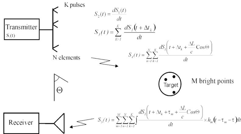
Fig. 1: The signal process.
