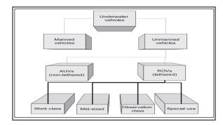
Figure 1 Underwater vehicles and ROVs
