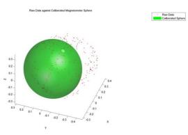
Figure 14 Comparison between calibrated data in green sphere against raw data
