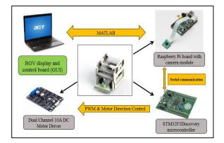
Figure 8 ROV overall system
