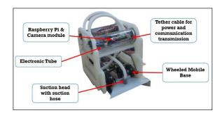
Figure 7 Actual design of ROV developed
