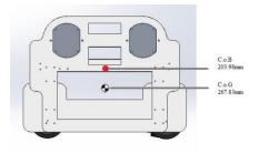
Figure 6 ROV center of buoyancy (C.o.B) and center of gravity (C.o.G)
