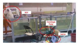
Figure 20 ROV underwater testing set-up
