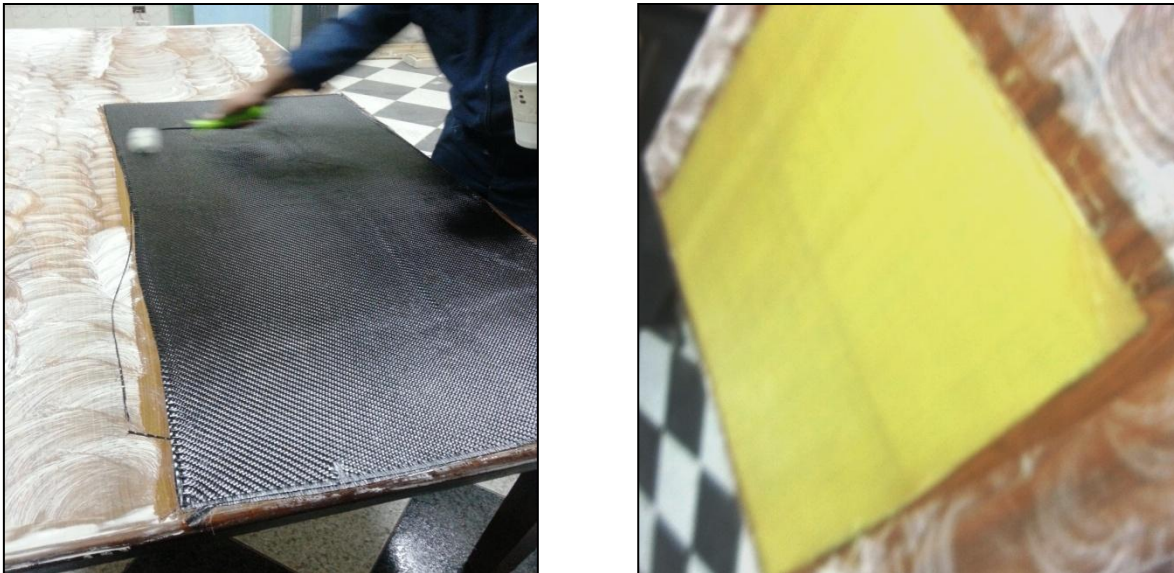
Fig. 1. Hand layup process for material fabrication
