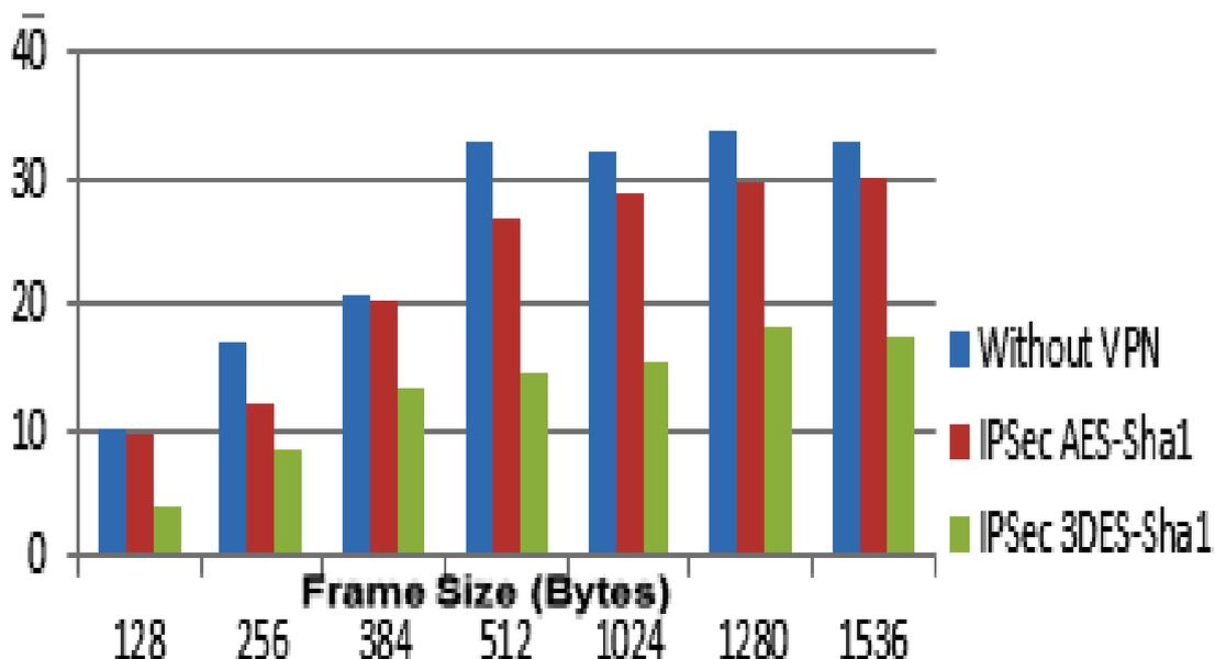
Figure 2 – IPsec VPN throughput results
