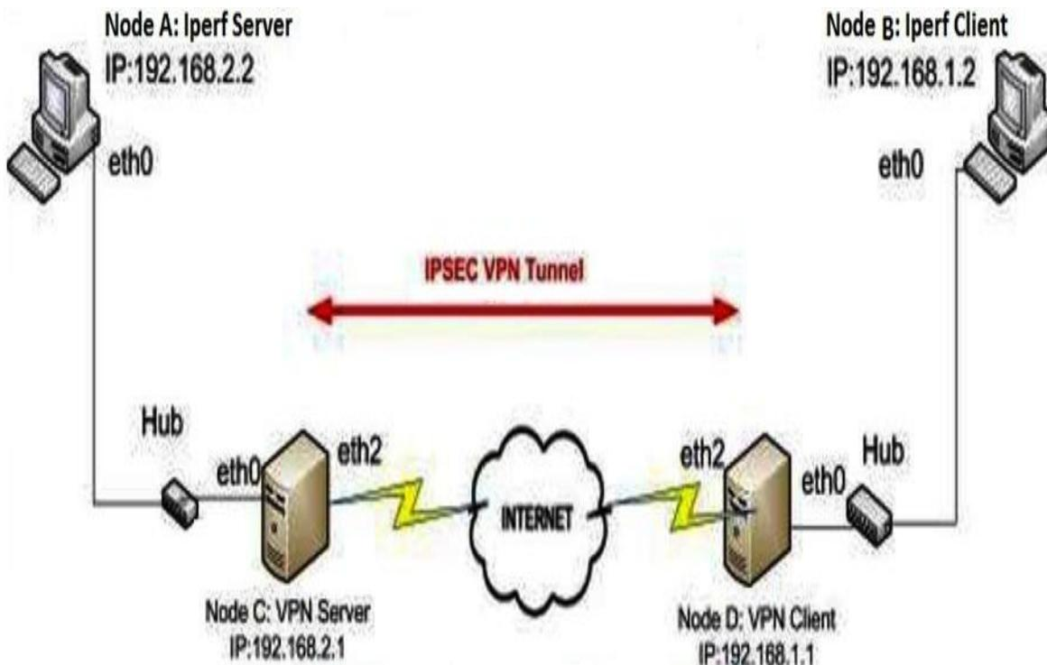
Figure 1 – Experimental Test-bed
