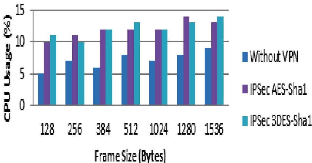
Figure 6 – IPsec VPN CPU usage results
