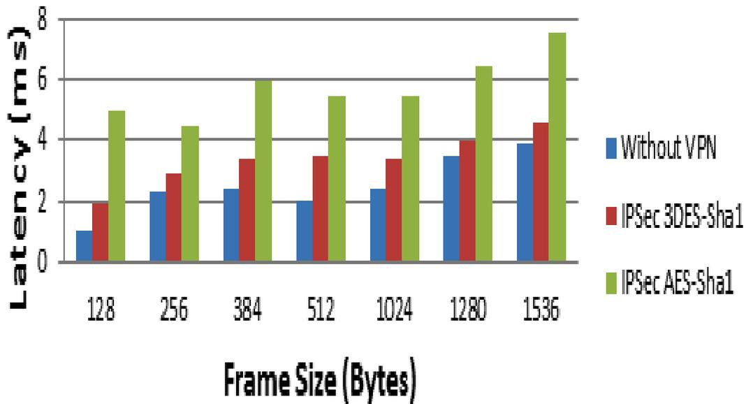
Figure 3 – IPsec VPN packet latency results
