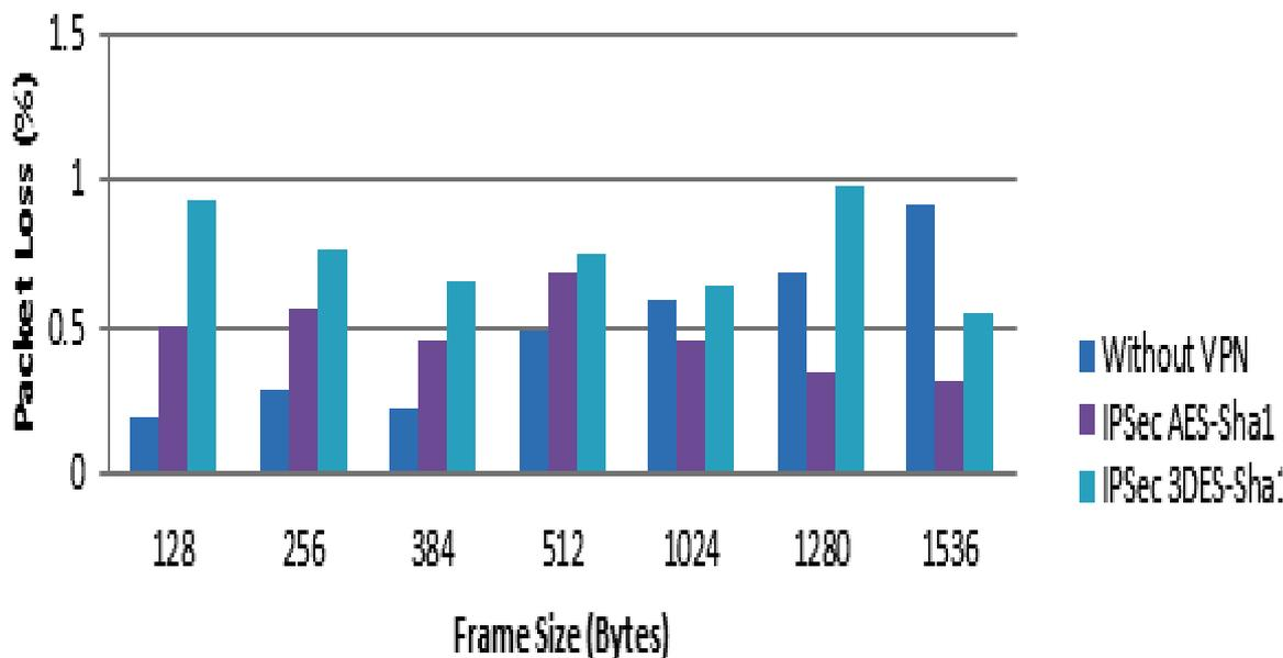
Figure 5 – IPsec VPN packet loss results
