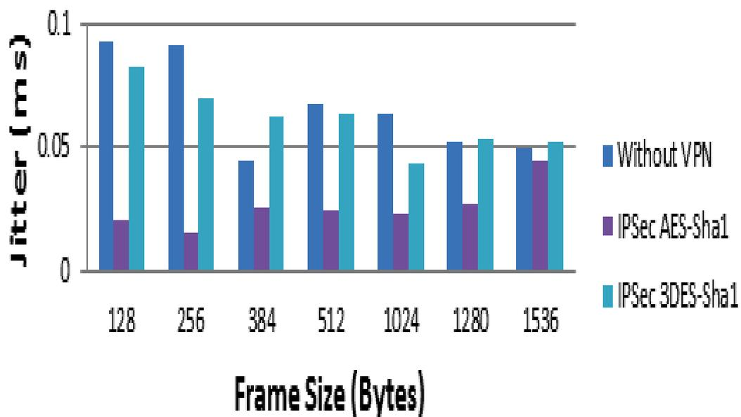
Figure 4 – IPsec VPN packet delay variation (jitter) results
