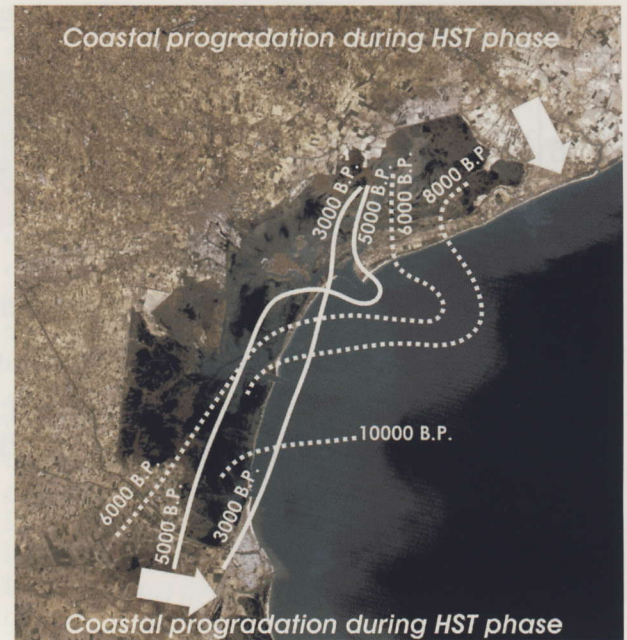
Fig. 12 – Model of Holocene evolution of coastline (from TOSI, 1994c, modified). Arrows: direction of advance of coastline, caused by progradation of river mouths during highstand tract stage.
