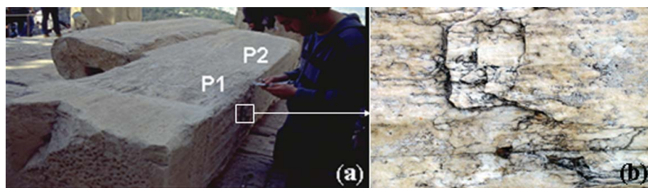
Fig. 1. The sampling site at the west side of the east wall of the Propylaea. (a) Collection of surface samples consisting of flakes, (b) Magnified view of the surface of the marble from which samples were collected (color figure available online).
