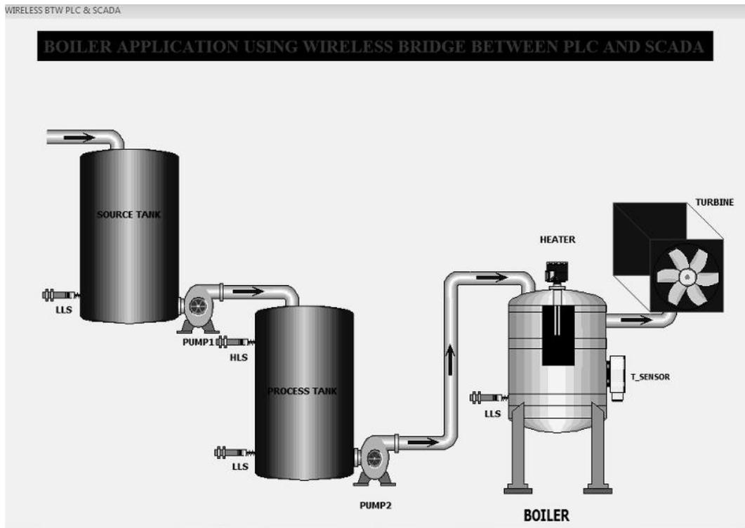
**Figure 6:** control of Boiler using SCADA
