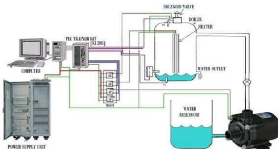
**Figure 1:** Diagram of boiler control using PLC
