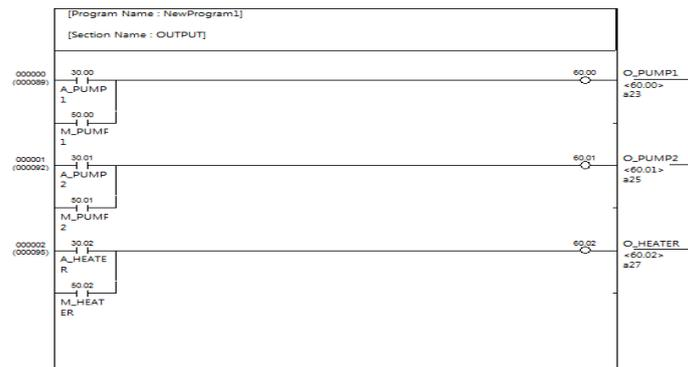
**Figure 4:** Manual page of ladder diagram output
