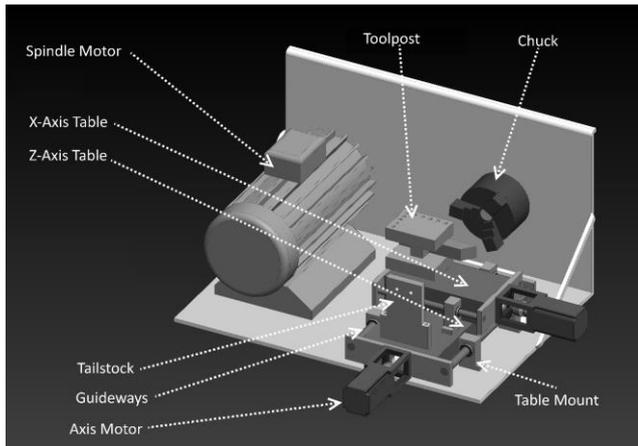
**Fig 2-9:** Dimetric View of our final CAD model with labels.
