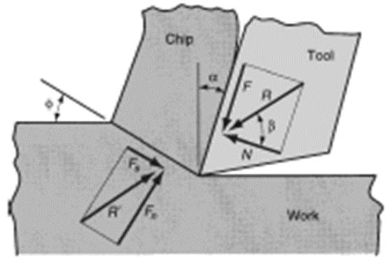
The Shear plane angle ( $\phi$ ) is further used in the merchant equation to get the value of  $F_t$ . There are *some assumptions that need to be considered before using merchant equation*:
