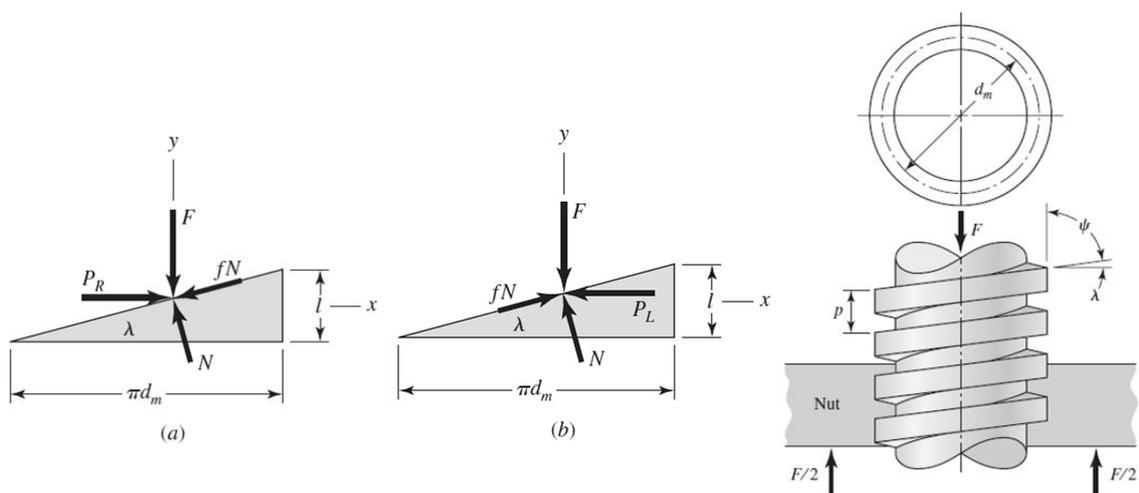
**Fig. 2.6:** Detailed Free Body Diagram of the Forces acting on a leadscrew.
