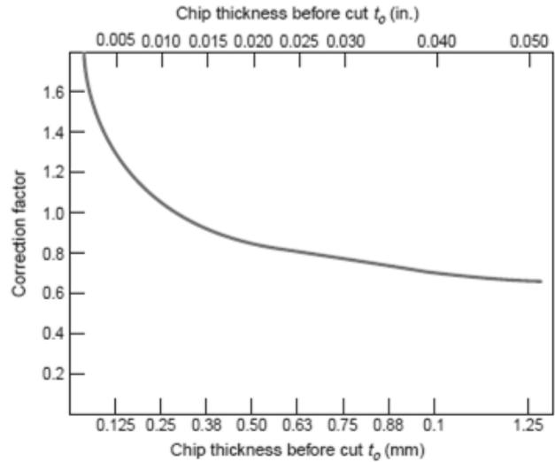
In the orthogonal cutting model, chip thickness before cut  $t_0$  is referred as feed of the turning operation. The graph above shows the correction factor to be applied for various feed operations.
