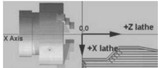
**Fig. 2. 4:** Top view of Lathe machine with axes' relation to the chuck visible.
