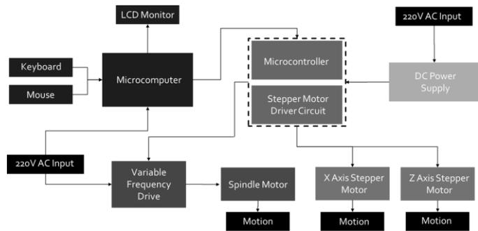
**Fig 4-6:** Schematic showing the complete electronic architecture of our machine.
