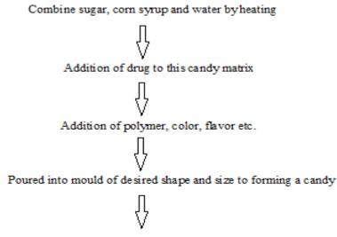
Sealing and wrapping of candy in polyethylene wrapping
