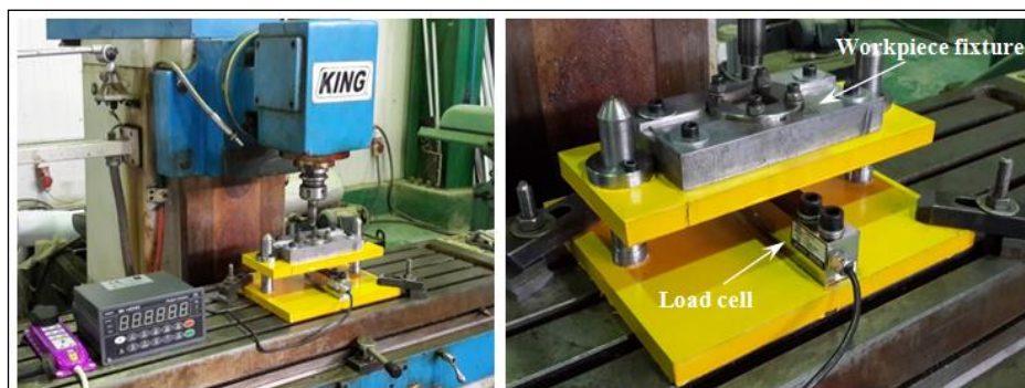
Figure 5: Axial load measuring rig.
