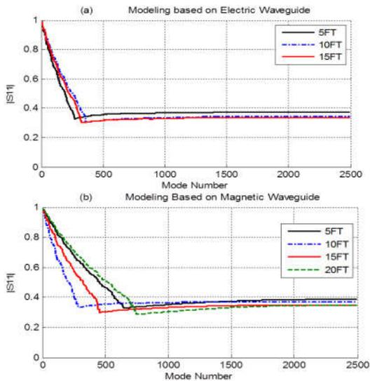
Fig. 5 S11 parameter as a function of mode number. (a) Modeling based on electric waveguide, (b) modeling based on magnetic waveguide.
