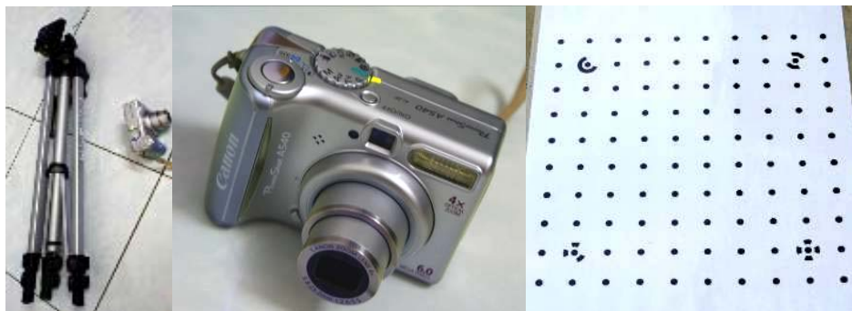
Figure 3. Devices used in camera calibration.
