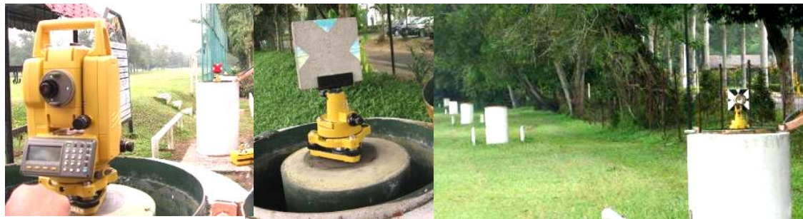
Figure 1. Instrumentations were used in total station calibration.
