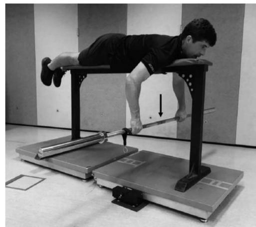
**Figure 2.** Bench pull perturbation set-up. Arrow denotes point of perturbation application.
