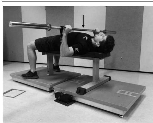
**Figure 1.** Bench press perturbation set-up. Arrow denotes point of perturbation application.
