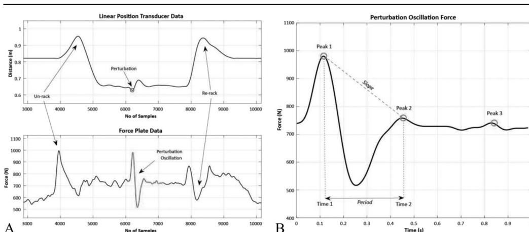
**Figure 4.** A) Linear position transducer signal used to determine perturbation onset. B) Peak identification to calculate natural frequency and stiffness.
