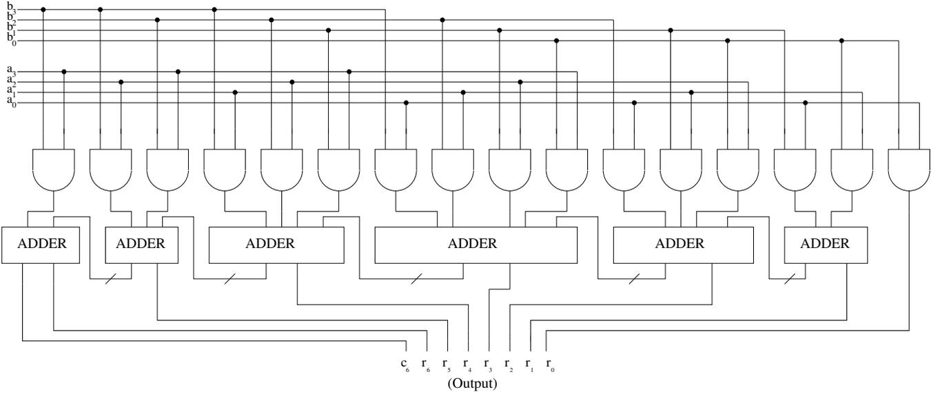
Fig. 4. Hardware Architecture of the proposed Vedic Multiplier.
