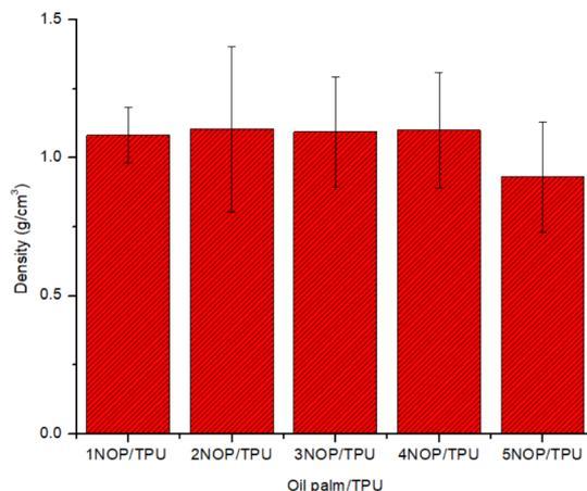
**Figure 3:** Density properties of nanocellulose oil palm/TPU.
