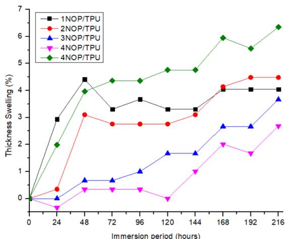
**Figure 2:** Thickness swelling properties of nanocellulose oil palm/TPU.
