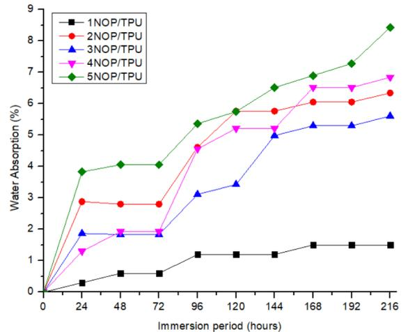
**Figure 1:** Water absorption of nanocellulose oil palm/TPU.
