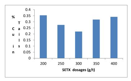
Figure 7: Grade of tailings at varying SETX dosages.
