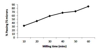
Figure 1: Milling curve for Palabora copper ore.
