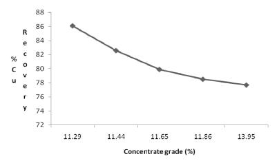
Figure 6: Relationship between recovery and grade of copper in concentrates.
