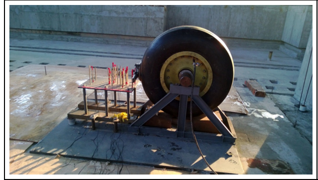
Figure 8. Apparatus of the jet blast field test system.
