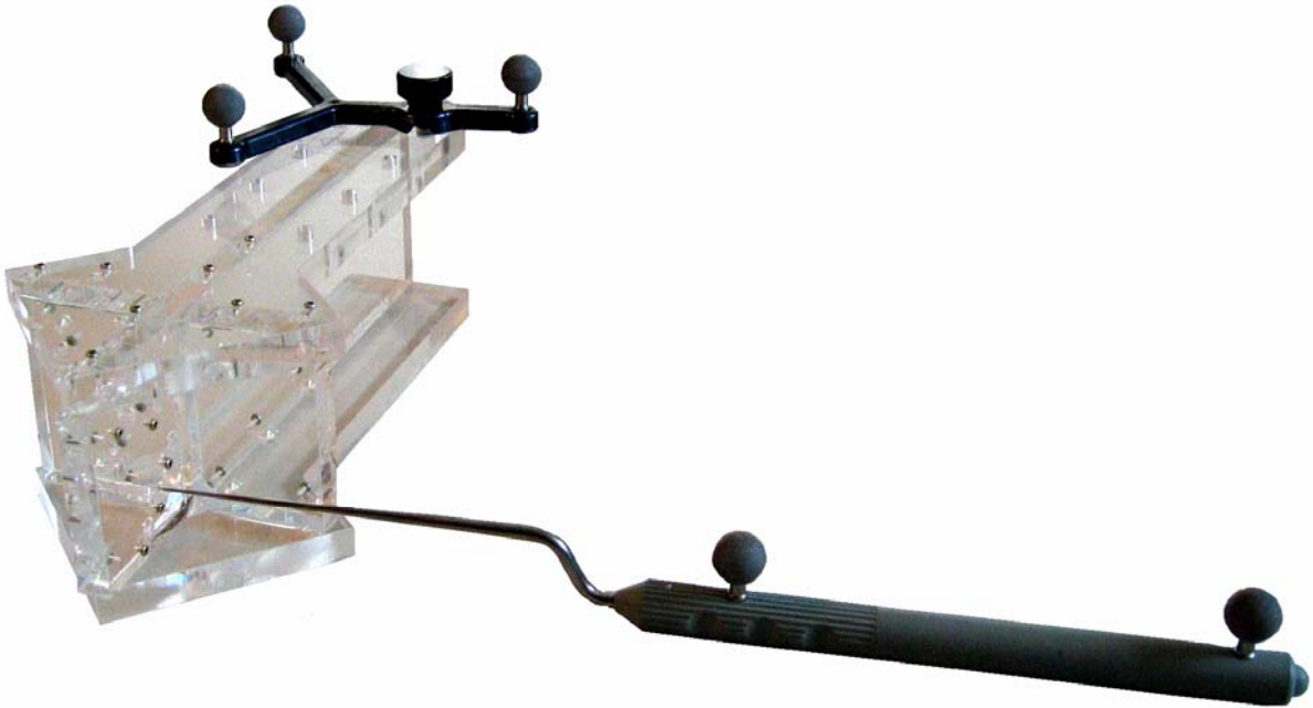
Figure 5 Accuracy measurement phantom consisting of a testing cuboid and a rack to attach the Laterostar. The navigated pointer is located in one of the inverted cone tips.
