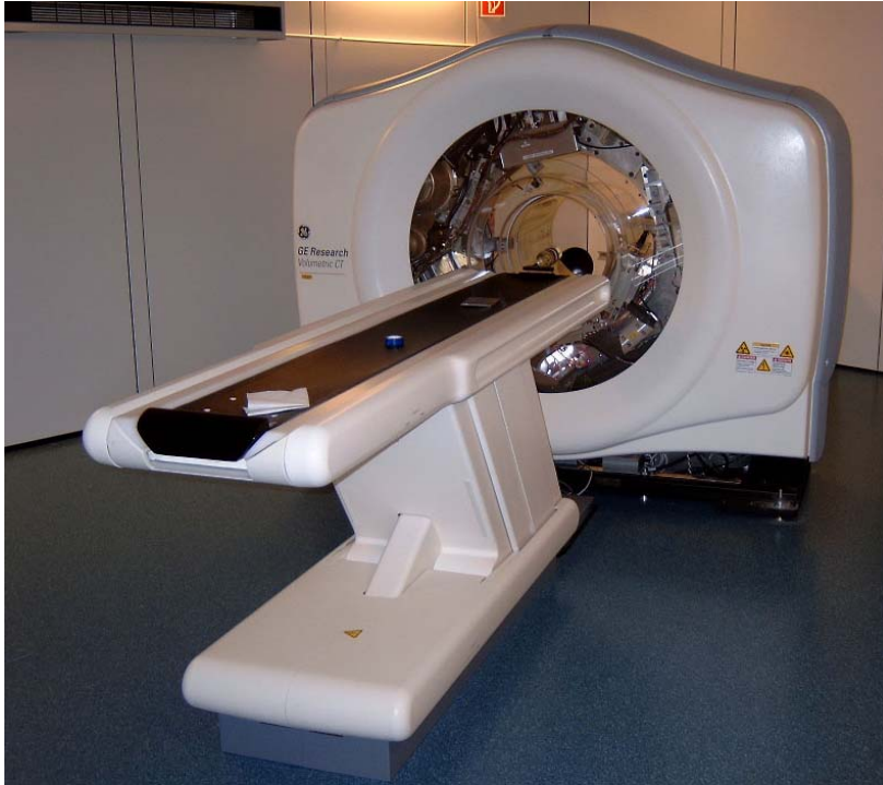
Figure 6 Flat-panel based Volume-CT prototype as used in this study. Despite the fact that from a technical view point scans of whole human skull base are possible, the machine is not approved for human scanning yet.
