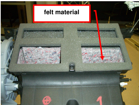
Figure 15 – Air Registers, face vents open and fitted with the felt material.
