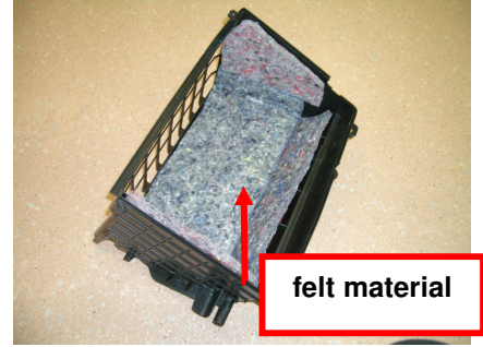
Figure 9 Inlet assembly, underside showing application of the acoustic felt.
