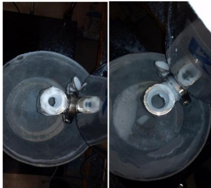
Figure 13: Picture of silicon dioxide buildup for (a) without static eliminator and (b) with static eliminator
