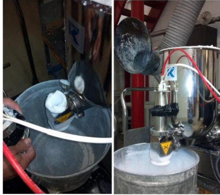
Figure 12: Picture of feeder (a) without static eliminator and (b) with static eliminator
