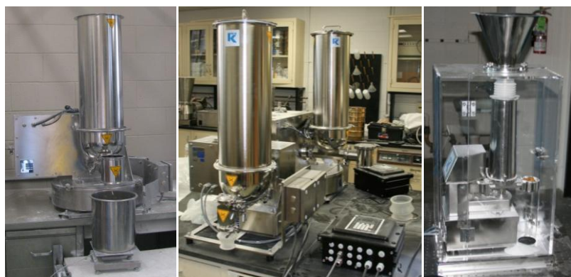
Figure 2: K-Tron KT35 feeder with Schenck Accurate AccPro II catch scale, K-Tron KT20 feeder, and K-Tron MT12 feeder.
