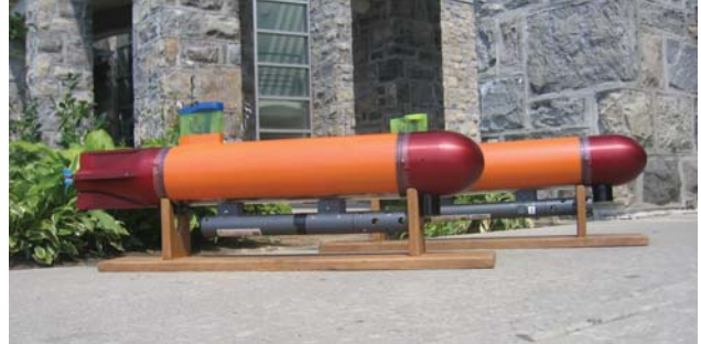
Fig. 1. Virginia Tech 475 AUV. The external payloads shown mounted below the vehicles were not used in the present work.
