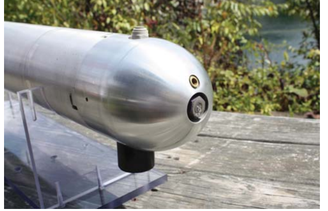
Fig. 4. Prototype nose showing galvanic release and vacuum ports.
