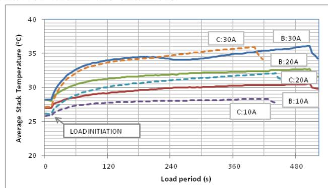
Fig. 6. The averaged stack temperature profiles at different loads for positive (B) and negative (C) cooling fan settings
