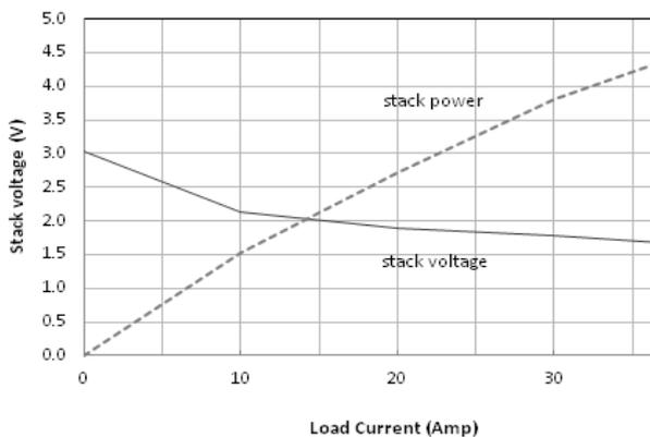
Fig. 4. Polarization curve of stack D1
