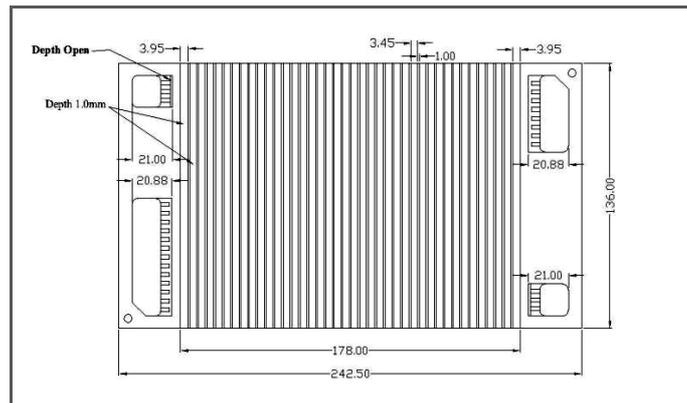
Fig. 1. The bipolar plate and cooling channel design geometry
