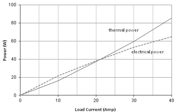
Fig. 5. Relation of electrical power to thermal power generation
