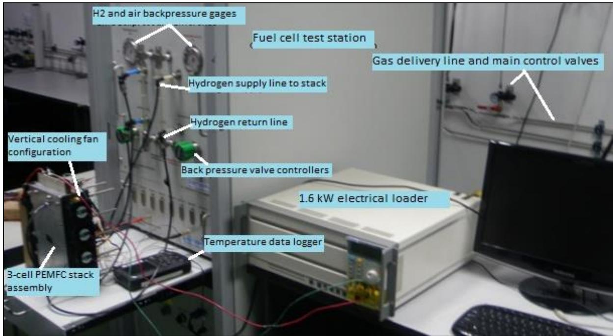
Fig. 3. Hydrogen fuel cell test station setup
