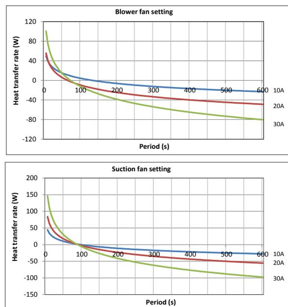
Fig. 7. Cooling profile for both suction and blower fan settings across all the loads
