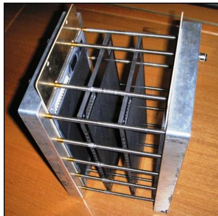
Fig. 2. Stack assembly displaying the integrated cooling channels within the two bipolar plates
