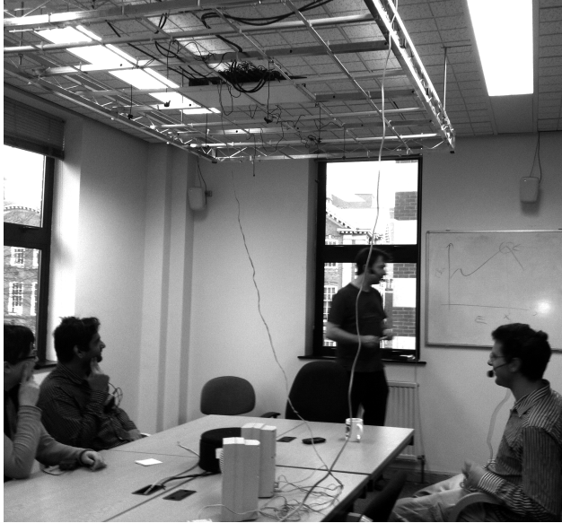
Figure 1: Meeting room recording setup. The boxes on the far wall are active-badge trackers. The frame on the ceiling and the black cylinder on the table each contain eight condenser microphones. Participants wear headsets and active badges.
