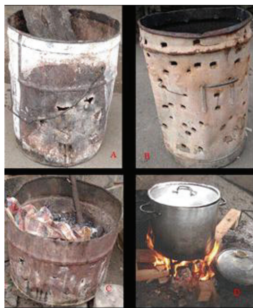
Figure 3: Biomass combustion technologies: (A) 20 litre imbaula ; (B) 70 litre dustbin type; (C) 100 l half-drum; & (D) 3-stone open fire place
