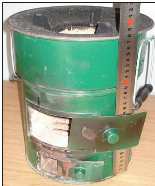
Figure 4: Image of GreenFire (Rocket) stove
