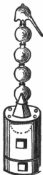
Fig. 11. Circular furnace with fractional distillation apparatus (Abraham Elezar pseud., from A. Crusius Erfurt 1735).
