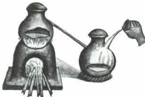
Fig. 4. Distillation apparatus using simple hand cooling for the receiver.
