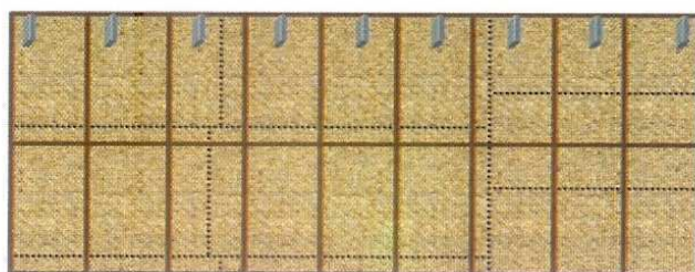
Fig.2. Graphical representation of the support, strainer and position of wooden blocks on wall as seen from verso
