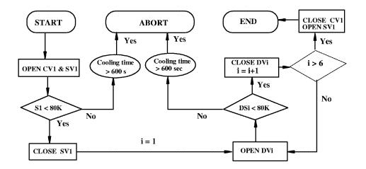
Figure 3. Simplified flow diagram of automatic filling system.
