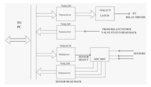
Figure 2. The block diagram of relay control, valve status and sensor read back.
