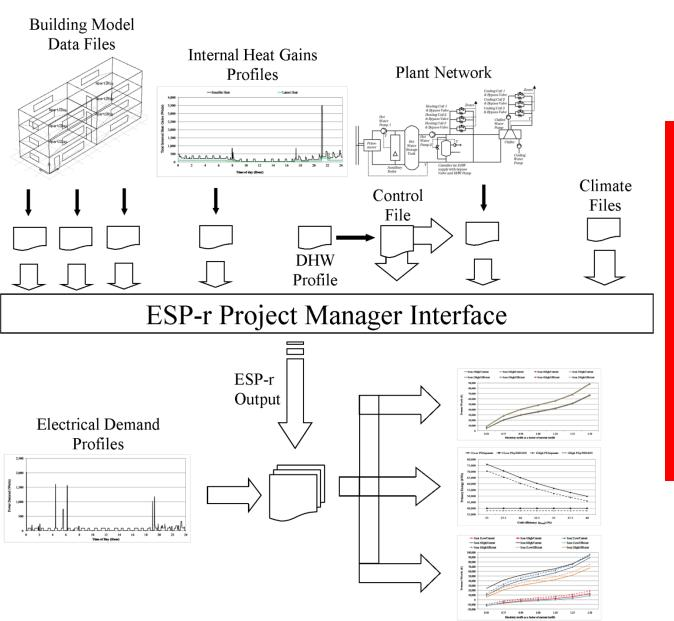
The building simulation tool ESP-r acts as the interface which permits the modelling of the supply side (the microtrigeneration system made up of multiple components) and the demand side (the user specified internal heat gains and building characteristics *etc.*)
