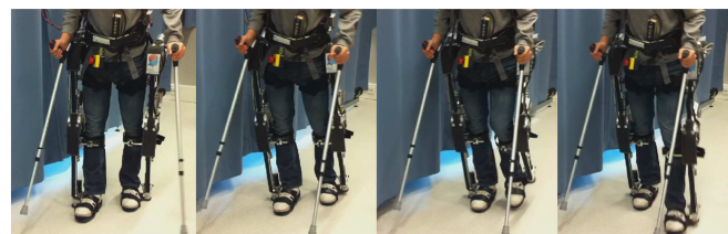
S5: double stance S6: assisted weight shift to right S8: full step left swing S9: double stance right foot leading left foot leading Fig. 10. Snapshots of a left step during straight walking. The crutches were only used for safety and did not touch the ground during the 8-meter walk.
