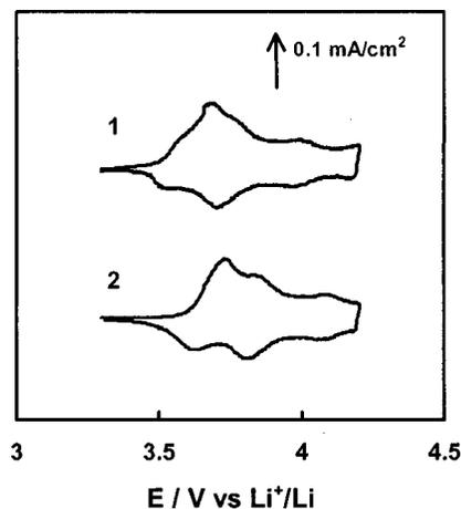
**Figure 5.** CV of the cathode in different electrolytes, which was recorded during the first cycle at a scanning rate of 0.01 mV/s. (1) 1 mol LiPF<sub>6</sub> 3:7 EC/EMC and (2) 1 mol LiBF<sub>4</sub> 3:7 EC/EMC.
