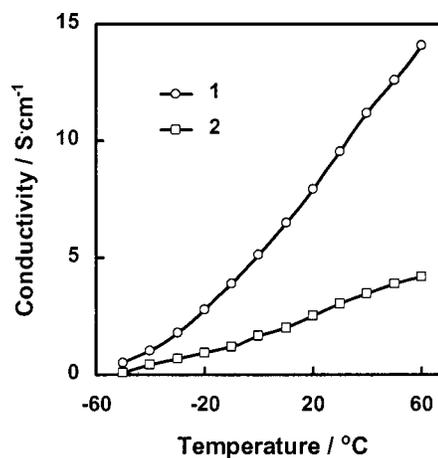
**Figure 2.** Ionic conductivity of the electrolytes as a function of the temperature. (1) 1 mol  $\text{LiPF}_6$  3:7 EC/EMC and (2) 1 mol  $\text{LiBF}_4$  3:7 EC/EMC.
