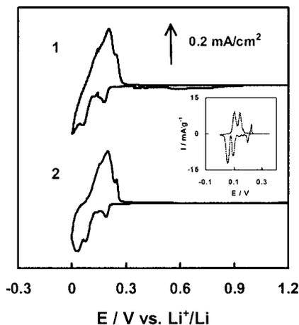
**Figure 3.** CV of the graphite electrode in different electrolytes, which was recorded during the first cycle at a scanning rate of 0.01 mV/s. (1) 1 mol LiPF<sub>6</sub> 3:7 EC/EMC and (2) 1 mol LiBF<sub>4</sub> 3:7 EC/EMC.
