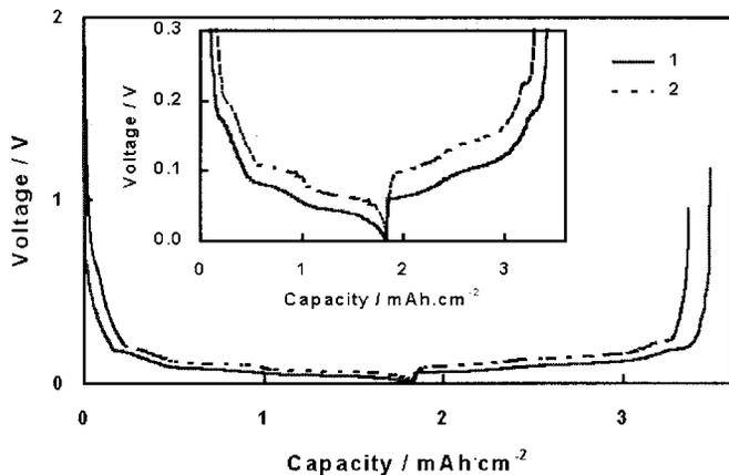
**Figure 4.** Voltage change of the Li/graphite cell with capacity in different electrolytes, which was recorded during the first cycle at a cycling rate of 0.5 mA/cm<sup>2</sup> between OCV and 0.002 V. Inset is a part selected from the voltage range of between 0.3 and 0.002 V. (1) 1 mol LiPF<sub>6</sub> 3:7 EC/EMC and (2) 1 mol LiBF<sub>4</sub> 3:7 EC/EMC.
