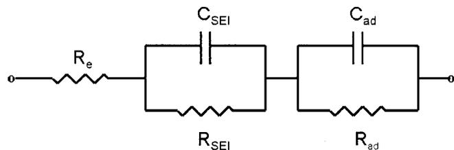
**Figure 10.** Equivalent circuit used for analysis of the impedance spectra.
