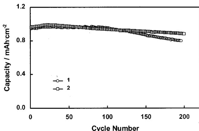
**Figure 6.** Discharge capacities of the graphite/cathode cells using different electrolytes at room temperature, which were measured at a constant current density of  $0.5 \text{ mA/cm}^2$  between 2.5 and 3.9 V with a taper of 20 min after charging voltage reached 3.9 V. (1) 1 mol  $\text{LiPF}_6$  3:7 EC/EMC and (2) 1 mol  $\text{LiBF}_4$  3:7 EC/EMC.
