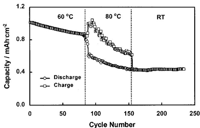
**Figure 8.** Charge and discharge capacities of the graphite/cathode cell vs. the cycle number at various temperatures. The electrolyte was a 1 mol  $\text{LiBF}_4$  3:7 EC/EMC solution with 80 ppm of water. Current density was  $0.5 \text{ mA/cm}^2$  and cutoff voltage was 2.5 V/3.9 V with a taper of 20 min after charging voltage reached 3.9 V.
