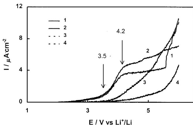
**Figure 1.** Response of passivation current of Al electrode to the potential in the electrolytes prepared by dissolving 1 mol lithium salt into 3:7 EC/EMC mixed solvent, which was recorded at a sweeping rate of 1.0 mV/s. (1) 1st sweep in  $\text{LiPF}_6$ , (2) 1st sweep in  $\text{LiBF}_4$ , (3) 2nd sweep in  $\text{LiPF}_6$ , and (4) 2nd sweep in  $\text{LiBF}_4$ .
