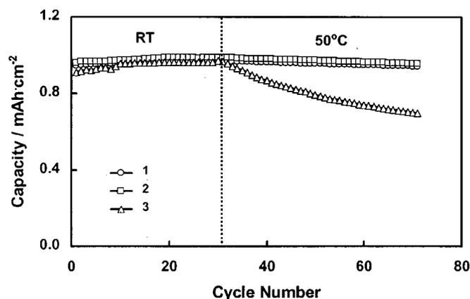
**Figure 7.** Discharge capacities of the graphite/cathode cells using 1 mol  $\text{LiBF}_4$  3:7 EC/EMC electrolytes with various water content, which were measured at a constant current density of  $0.5 \text{ mA/cm}^2$  between 2.5 and 3.9 V with a taper of 20 min after charging voltage reached 3.9 V. (1) 22 ppm, (2) 80 ppm, and (3) 620 ppm.
