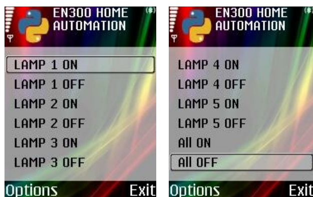
Figure 5. Cell Phone GUI for controlling the home appliances
