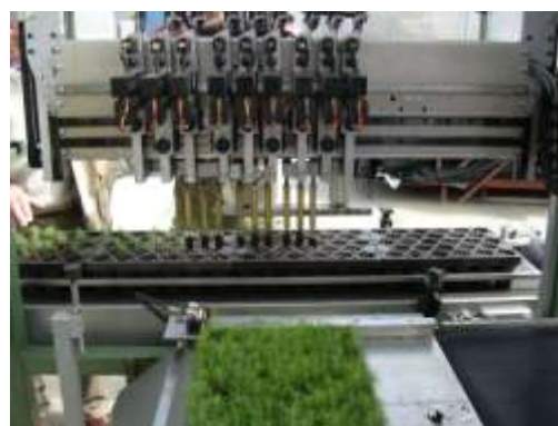
Figure 4. The grading and re-plug robot designed in the PRE-FOREST project.
