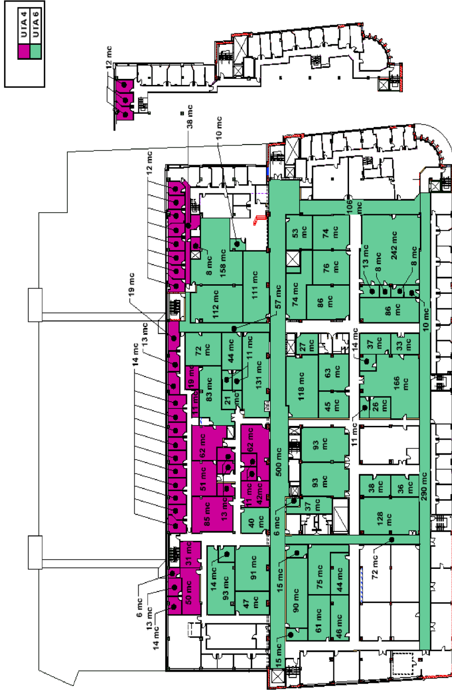
Figure 1. Schematic of zones at second floor served by AHU-6 and AHU-4 units.
